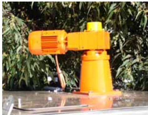
gear driven mixer with bevel helical gear unit on a closed top vessel at atmospheric pressure
