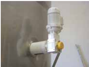
3.0 kW Side entering Mixer Dairy Food Production
