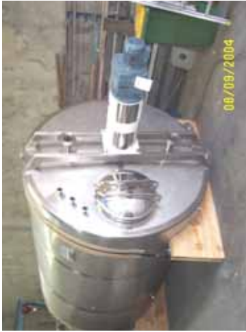
Series 70 mixer 30,000 litre slurry holding tanks
