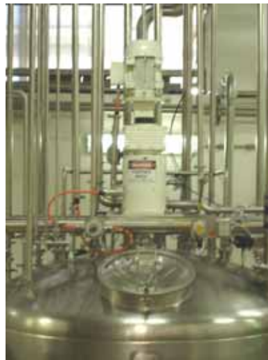
series 75 mixer, 11kW, gear driven
