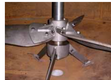
tripod style steady bearing with bronze bushing
