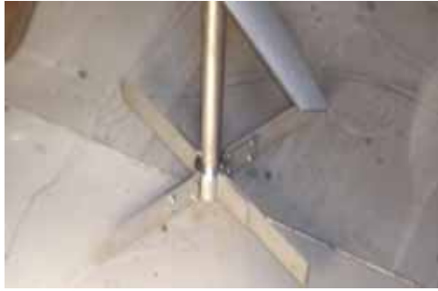
radial flow impeller on bottom of tank type "RF"
