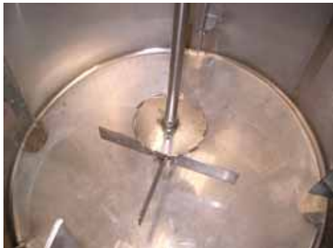
radial flow on bottom, dispersion disc on top type "RF" + type "DD"
