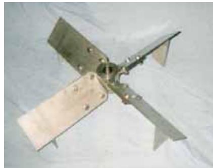
pitched blade turbine with stabiliser fins and bolt on blades
